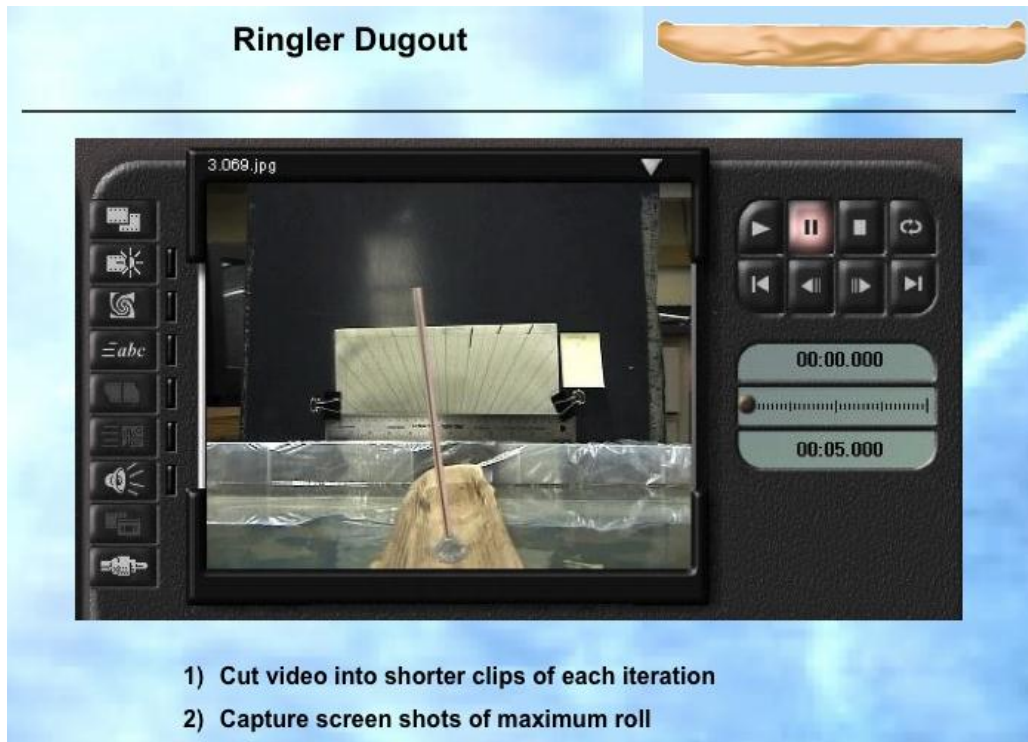
Figure 11. This photograph taken by William Wright shows the video equipment (on each side of the image) that was used to visually record changes in the rolling angle of the dugout under various loads. The center of the image is a still from the video showing the dugout and the needle arrangement for marking a roll angle. The entire video was played later and the angle readings recorded for use in calculating graphs such as the one in Figure 12.
